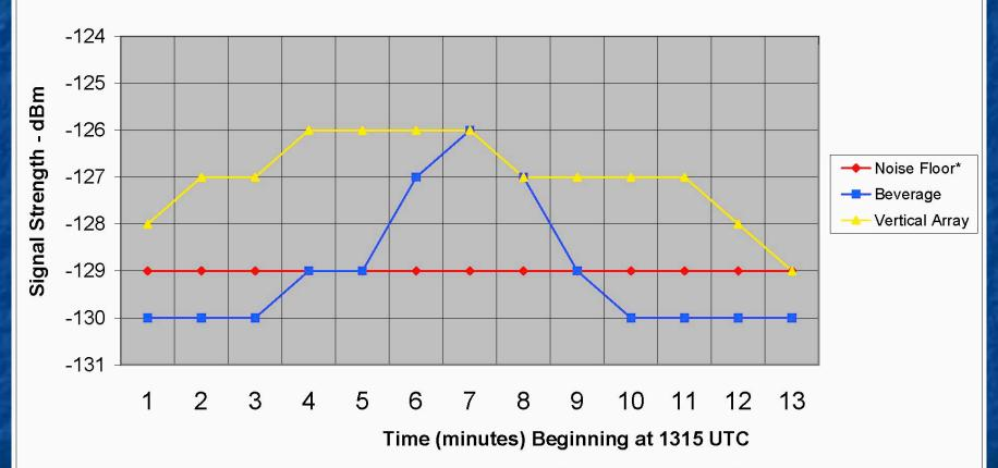
\*Average Noise Floor - Actual is Beverage -128 dBm / Vertical Array -130 dBm. Signal levels shown below the noise floor are only to indicate signals not copyable and are not measurements
