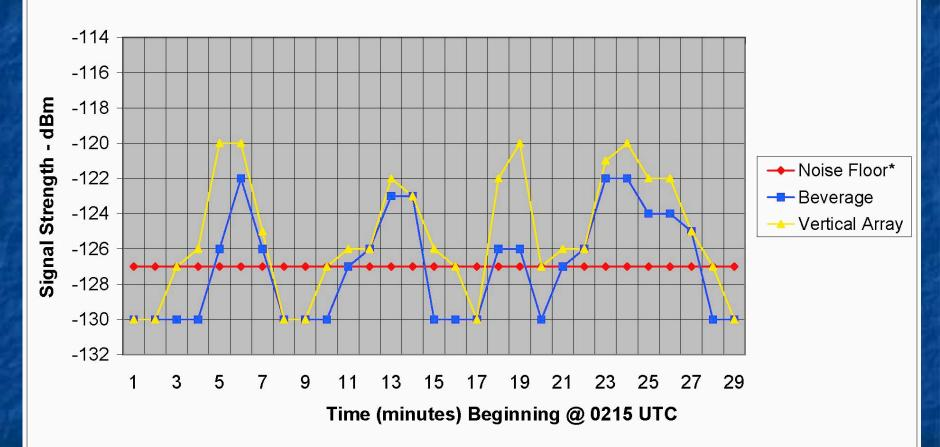
\* Noise Floor Average - Actual is Beverage -125 dBm / Vertical Array -129 dBm. Signal levels shown below the noise floor are only to indicate signals not copyable and are not measurements
