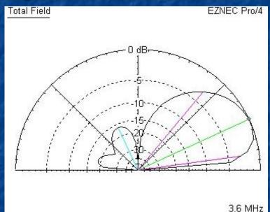
Elevation Plot Cursor Elev 25.0 deg. -4.56 dBi Azimuth Angle 90.0 deg. Gain Outer Ring -4.56 dBi 0.0 dBmax 0.0 dBmax3D 3D Max Gain -4.56 dBi Slice Max Gain -4.56 dBi @ Elev Angle = 25.0 deg. Beamwidth 42.8 deg.; -3dB @ 7.8, 50.6 deg. Sidelobe Gain -20.77 dBi @ Elev Angle = 115.0 deg. Front/Sidelobe 16.21 dB
