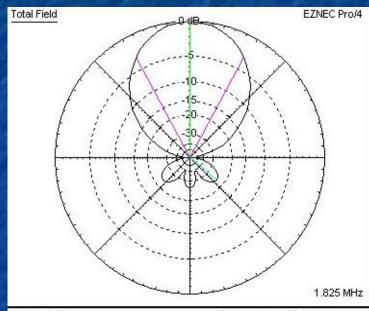
Azimuth Plot Cursor Az 90.0 deg. Elevation Angle 25.0 deg. Gain -11.21 dBi Outer Ring -11.21 dBi 0.0 dBmax 0.0 dBmax3D
