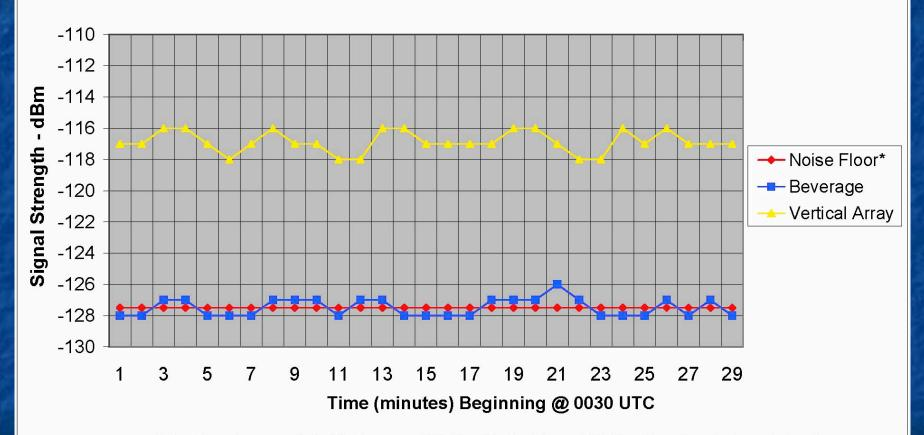
\*Noise Floor Average - Actual is Beverage -125 dBm / Vertical Array -130 dBm. Signal levels shown below the noise floor are only to indicate signals not copyable and are not measurements
