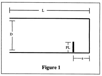
affect this distance, most notably diameter and length of the horn. My experience has been to place the radiating element about  $0.4\lambda$  from the closed end.
