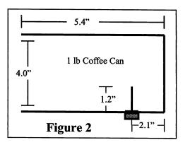
purchase brass strips at a local hobby store. The tubing will slide over the N center pin. Al Ward prefers to use two pieces of tubing, one smaller than the other. The smaller piece to be soldered to the center pin and the other telescoping over and soldered to the smaller one. This will allow increasing or decreasing the length of the probe for tuning.
