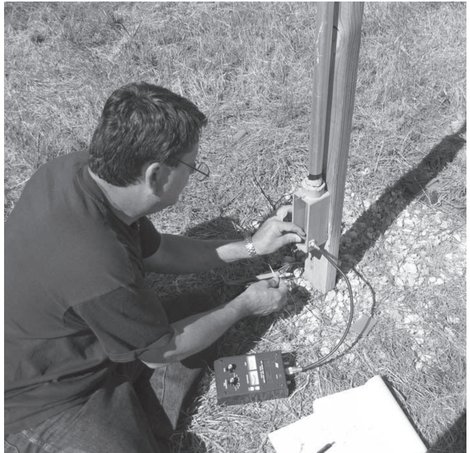
Figure 20 — W5ZN measuring the self-resonance of the vertical elements.
