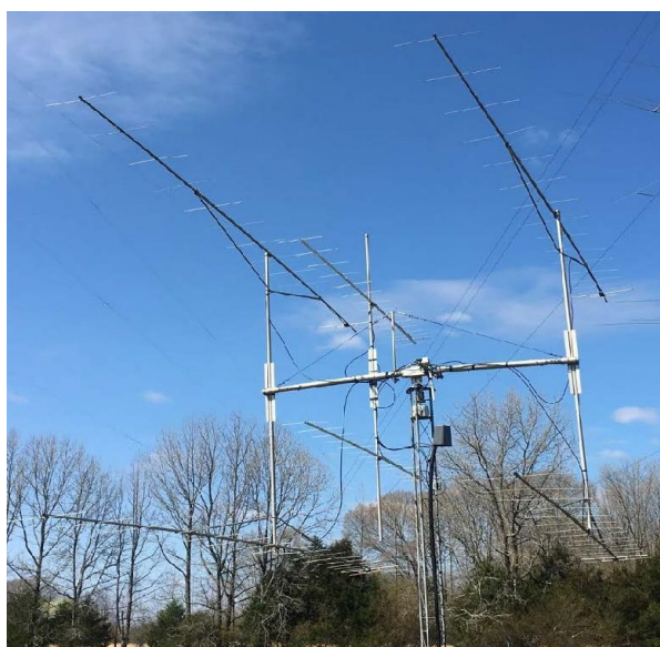
W5ZN 2xFO16 222 MHz EME Array
